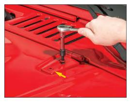
ratchet. (it may be necessary to score the paint around the bolts using and razor blade to prevent paint chipping.)
