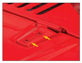
Put on Safety Glasses. With the hood securely latched in place, locate the two T47 Torx bolts on both hood hinges and remove them using a T47 Torx bit and
