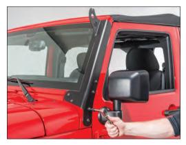
Place the bracket over the hinge plate and align the holes on the bracket with the holes in the factory hinge plate. Reinstall the 6 T40 torx bolts lightly with at T40 torx bit and ratchet but do not fully tighten at this time.
