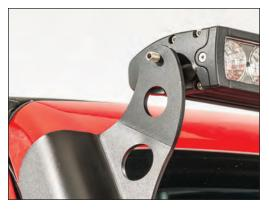
spacer on both ends. Carefully insert the stud through the hole in the bracket on the passenger side.
