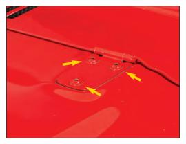
Put on Safety Glasses. With the hood securely latched in place, locate the three T40 Torx bolts on both hood hinges and remove them using a T40
