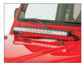
Adjust lightbar to the desired angle, then and tighten the nuts with a 13mm wrench.
