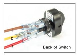
Connect the wires to the interior switch (G) as shown: (I) brown (ground/earth) to the top post. Yellow (D) (trigger wire) to the center post. Red (J) (positive from outlet harness) to the lower post.
