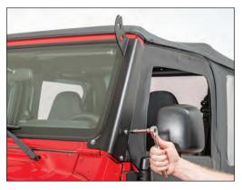
Place the driver side bracket against the A pillar and attach using 3 supplied hex head cap screws and washers.
