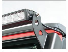
Install washer, split washer, and nut (supplied with lightbar) on both sides. Adjust lightbar to the desired angle, then and tighten the nuts with a 13mm wrench.
