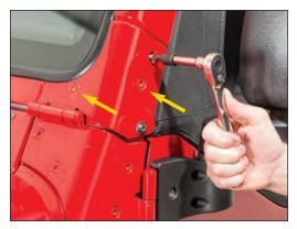
Put on Safety Glasses. Locate and remove the 3 T40 torx bolts from the upper windshield hinge.
