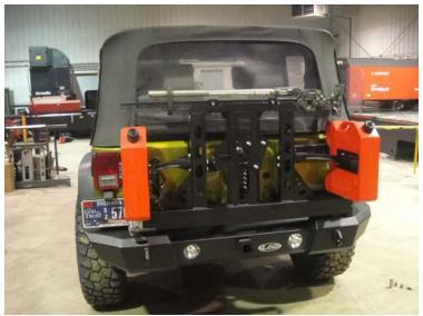
3. Repeat the first two steps for the other side. **Note:** If your tire carrier is our door-linked version then the driver side can mount will not bolt to it. Only the passenger side mount can be used with the door-linked version.
