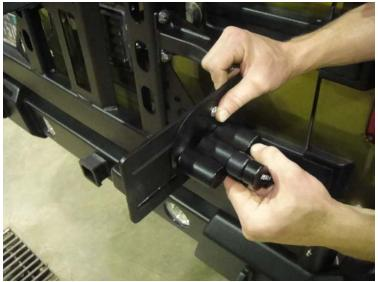
3. Place the Roto-Pax mount against the arm. This mount is also adjustable forward and back. This allows the cans to be mounted as close to the body as possible.
