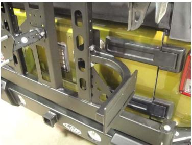
1. Place the arm up against the tire carrier. Bolt the arm to the carrier frame using two (2) 3/8" x 1" bolts per side. There are many height positions to choose from when mounting these. **Note:** The center of the main arm that comes around will be the center height of these gas cans.
