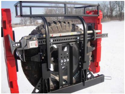
2. Set the rack on top of these arms and place the four (4) 5/16" x 1" bolts down through the rack and tabs on the arms. Once all four bolts are in place (don't tighten these bolts yet), move the rack so that it sits level to the ground and tighten the arms where they mount to the tire carrier. Than go back and tighten the four bolts holding the rack to the arms.
