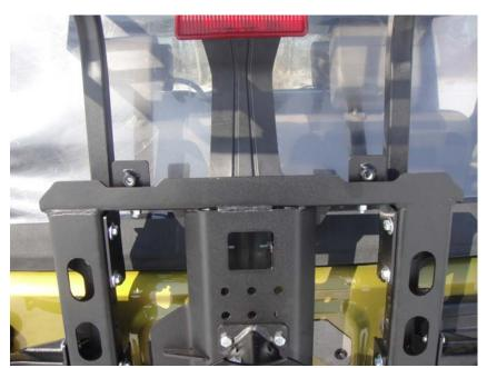
1. Begin with mounting the square tube arms to the carrier system. The arms must be bolted to the inside of the carrier uprights. The flat plates of these arms are the bottom side and are what needs to be bolted to the carrier. The height of these arms will set the height of the rack. Use the four (4) 3/8" x 1" bolts to mount these arms. Do not tighten these bolts until after bolting the rack to the arms.
