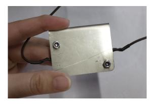
**6.** Align and attach the provided Tinnerman S-clips on resistor mounting bracket. The rounded edge should be on the same side as the resistor. Leave about 1 inch of space between clips.
