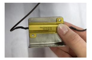
**5.** Secure the nut on the back of the resistor mounting bracket with a pair of pliers OR adjustable wrench, then tighten both screws with a Phillips screwdriver.
