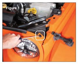
Put on safety glasses. Prepare the vehicle by removing the outer two grille retainer pins. Depending on model year, pry up or unscrew the plastic fasteners using a small screwdriver. Early model vehicles may feature Phillips head
