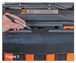
Mark the grille to hood weather stripping where the deflectors tab rests. (see FIG 3)
