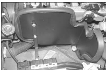
10. Using the provided hardware secure the "L" bracket to the inner fender as shown. Now tighten all hardware.
