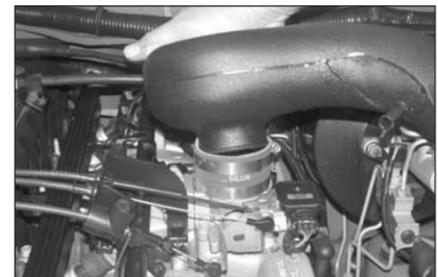
12. Install the K&N intake tube into the silicone hose on the throttle body.
