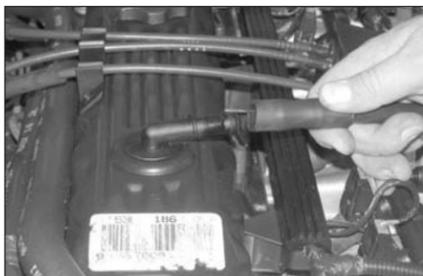
3. Disconnect the crank case vent line at the valve cover.
