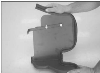
7. Install the trim seal to the heat shield as shown. Trim as needed.
