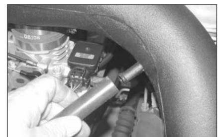
14. Connect the other end of the silicone hose to the vent on the K&N intake tube.
