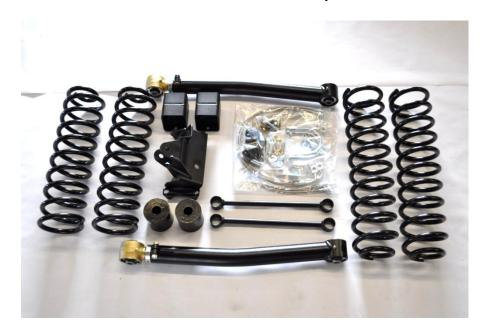
NOTES: Cutting and grinding is required to complete the installation of the rear roll center correction trackbar bracket. Wheel spacers or aftermarket wheels with a smaller backspacing than factory (4.5" or smaller number are recommended) are required for a complete installation. Aftermarket CV drivelines are recommended. Welding on rear trackbar bracket is recommended after installation.
