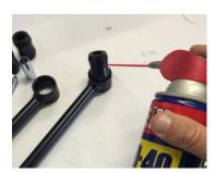
43. Install Swaybar bushings into supplied swaybar links, use of a lubricant and a small hammer will assist in this process, install swaybar endlink tubes into swaybar bushings. Install
