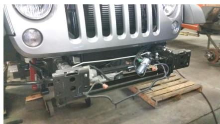
Install EVO Pro Series Winch Plate. Slide the EVO winch plate in between the factory frame rails as shown. Angle the winch plate as you slip it into
