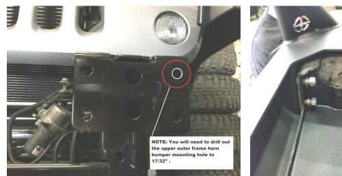
through the EVO winch plate, then securing it to the factory front frame horns with the included  $\frac{1}{2}$ " washers and  $\frac{1}{2}$ "-20 stover lock nuts. Torque to 85 ft/lbs.
