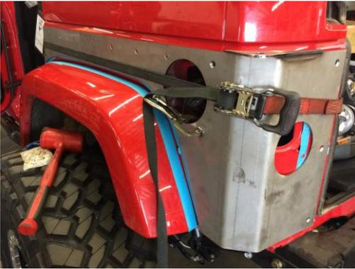
5. Use a large C-clamp through the rear taillight hole in body and clamp RockSkin to body.
