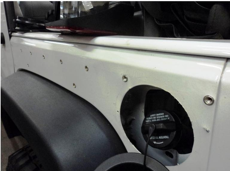
9. Install nutserts into drilled holes. Fully thread the long 1/4" bolt with nut into the nutsert as seen in photo. With wrenches hold the bolt stationary and turn the nut 2 - 3 turns making sure that the nutsert does **NOT**
