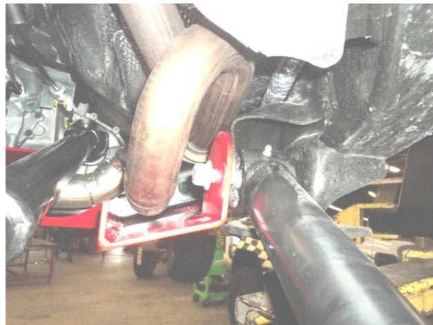
1. Remove factory transercase skid (4 bolts: 2 on the center of the transmission cross member, 1 on gas tank, 1 on driver side frame)
