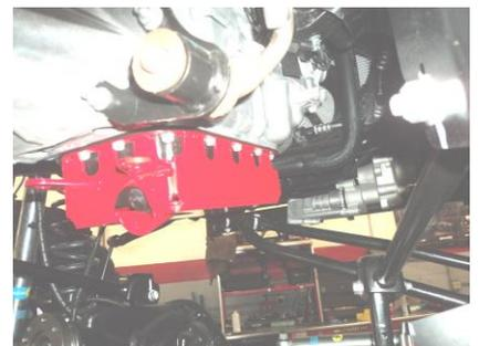
7. With all bolts just slightly touching the EVO Skid, begin to tighten all bolts in a crossing fashion to 85 **in/lbs**. The pan/skid will work its way to become tight and compressing the RTV sealant. You will need to go over all bolts in this crossing fashion a few times until all bolts are tight.
