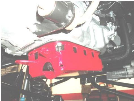
begin to touch the EVO Skid. **VERY IMPORTANT: Do not fully tighten any bolts/nuts at this stage.**
