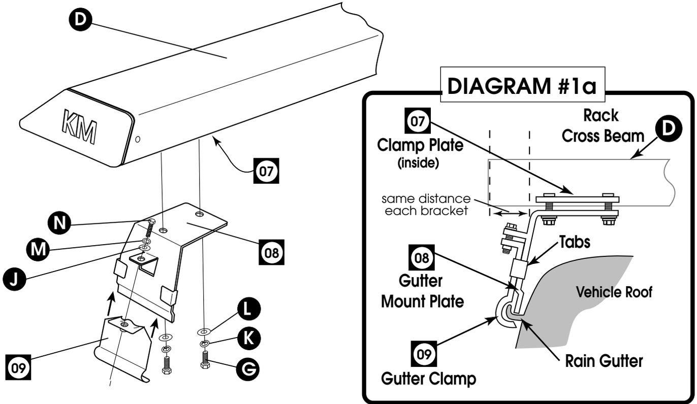
**#1**=Align mount plate holes with clamp plate holes (in cross beam) and attach gutter mount plates **08** with bolts **G**, lock washers **K**, and flat washers **L**, finger tight so mount can easily slide on cross beams.
