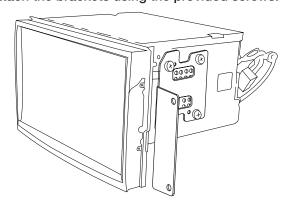
5 Run the key harness through the top-left side of X009 headunit. Mount the X009 headunit using 4 x 7mm factory screws.
