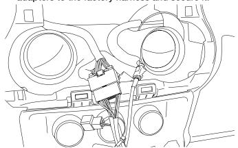
4 Place GPS antenna next to the instrument panel as illustrated and run the cable to the radio cavity.
