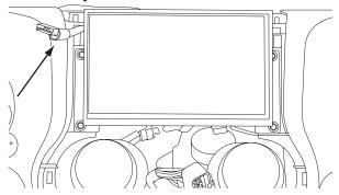
6 Connect the radio bezel and snap it into place.
