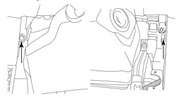
3 Remove the window switch pod using a panel removing tool and extract 1 x 7mm screw.
