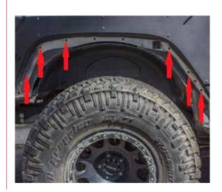
Install the Nutsert into the holes that you just drilled. It is good practice to paint the new holes or use RTV on the Nutsert to stop any rust from forming at the drilled holes. For further instructions on installing the Nutsert please refer to the separate install document.
