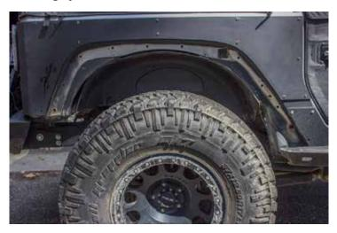
4 With the rear fender off, you can now mark and trim the inner fender liner. We recommend using the body line as your guide.
