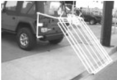
Rack in most downward position for installation/ removal of hardtop
