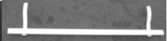
Rear pivot support 3/4" X 1 1/2" rectangular tube 51 3/8" long
