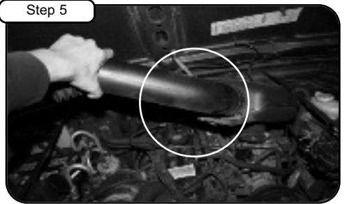
Pull crank case line away from stock intake and remove from vehicle.
