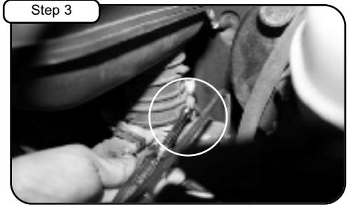
Loosen clamp on throttle body using 5/16" nut driver.
