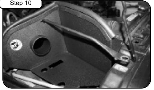
Attach trim seal to housing and install. Make sure core support bracket slides through hole on housing.
