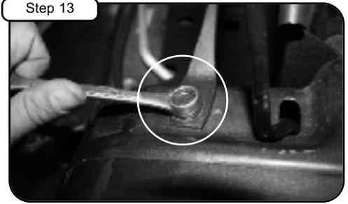
Secure core support bracket using 13mm.
