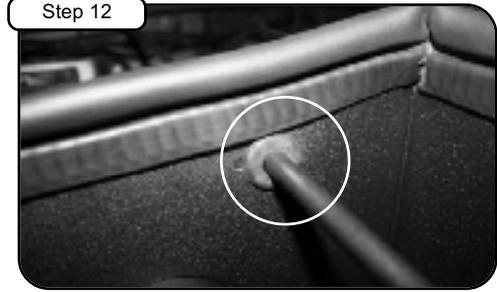
Align grommet from step 8 and position in hole to prevent core support bracket from vibration.
