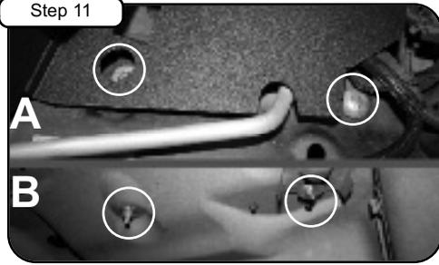
**A) Top view:** Secure housing using hex screws, fender washers, wavy washers and nuts. **B) Bottom view:** Tightening using 10mm socket or wrench.
