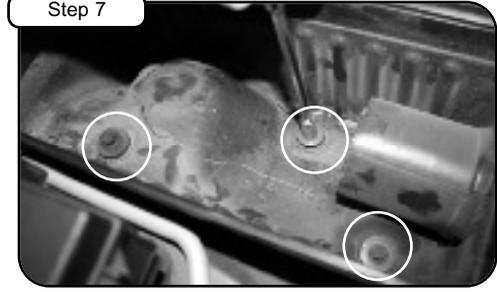
Remove upper half of air box. Loosen the 3 bolts on bottom of air box using 8mm socket or wrench and remove.
