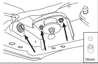
Using a 15mm wrench assemble steel bracket to Linkage assembly. Torque bolts to 20 ft-lbs.
