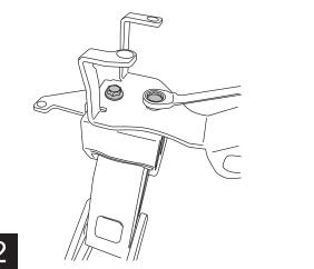
Drop threaded plate into slot in frame. Slot is located on both sides of the frame. The outer slot is preffered but may not be accessable with aftermarket bumpers or racks.
