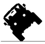
Modifying your Jeep® to improve off-road performance may result in vehicle handling different than as factory equipped, including increased ride-height and/ or chassis articulation; reduced lateral stability and higher risk of roll-over or other accident. Also, owner's choice of larger tire and wheel combinations may require additional braking force or increased stopping distances.
