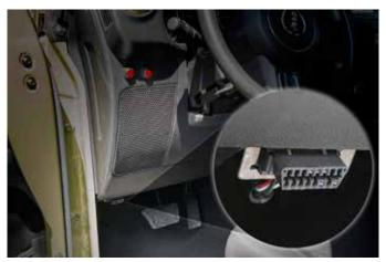
Note: Do not remove the programming cable during any programming sequence. If you do, the vehicle may not start. A JKS J-CAL programmer is designed to automatically go into Vehicle Recovery Mode and if this occurs, it will return your vehicle to stock.
