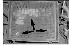
5. Loosen and remove the three bolts that secure the lower air cleaner assembly.
