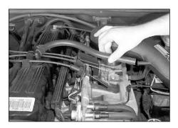
16. Install the provided silicone hose onto the crankcase vent on the valve cover, then install the other end onto the K&N intake tube.
