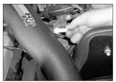
17. Install the 1/4 x 3/8" vent fitting onto the K&N intake tube as shown. **NOTE**: some earlier models may not be equipped with an EVAP canister, use the 1/4 plug provided and install onto the K&N intake tube.
