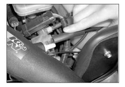
19. Install the new silicone hose onto the EVAP canister vent line and install the other end onto the K&N intake tube as shown.
