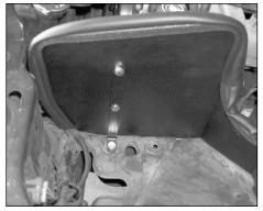
12. Install heat shield assembly into vehicle as shown. Using the hardware provided, secure large "L" bracket onto vehicle inner wheel well.
