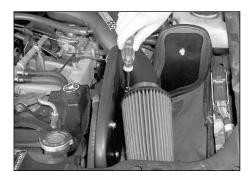
20. Install the K&N Filtercharger onto the K&N intake tube, then adjust the intake tube for best fit then tighten all hardware.
