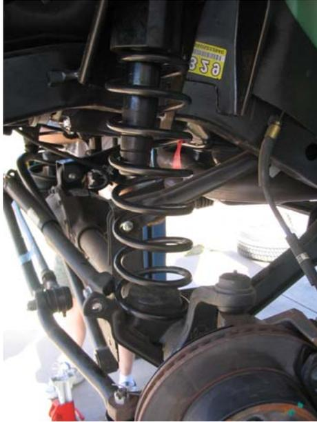
11. Now that the coil springs are installed go ahead and install your lifted front shocks( not supplied.) and raise up the axle and connect the sway bar end link and track bar to axle mount.
