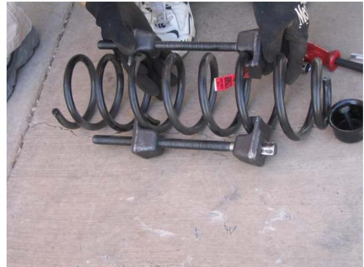
10. Once the coil spring is compressed , install it in the Jeep over the spring spacer.
