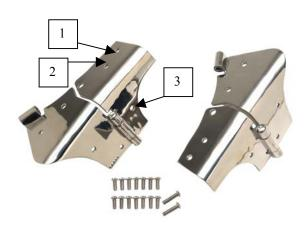
Note: The factory bolts have been installed using a thread locking cement, and sometimes are difficult to remove unless heat is applied to the head of the bolts. The factory has also put a threaded back-up steel plate inside the windshield to accept the bolts, this plate could fall inside the windshield.
