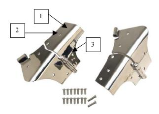
Note: The factory bolts have been installed using a thread locking cement, and sometimes are difficult to remove unless heat is applied to the head of the bolts. The factory has also put a threaded back-up steel plate inside the windshield to accept the bolts, this plate could fall inside the windshield.
