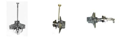
Place a very small screwdriver in the square hole at the top of the key lock mechanism. Push down on the retaining clip while pulling on the cylinder of the key lock.
