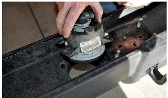
Install the factory fog lamps into the fog lamp mounts in the back side of the Brawler™ Front bumper. Re-use the OE retaining screws. These sheetmetal screws will form their own threads as you drive them into the retaining rings on the Brawler bumper, so press firmly as you twist the screwdriver.
