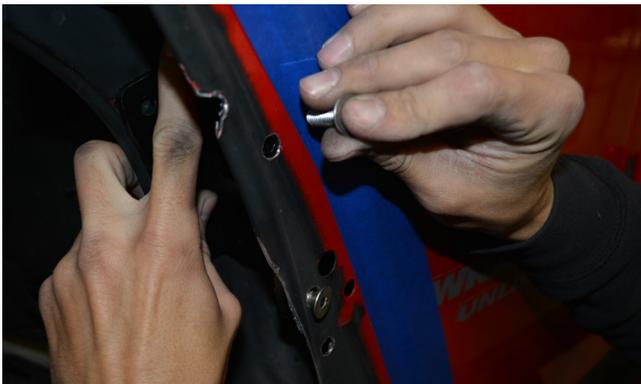
**17. With the Lower Sub-Frame Bracket** temporarily in place, use the fine-tip felt marker to mark the two hole locations in the inner tub brace. Then remove the bracket.
