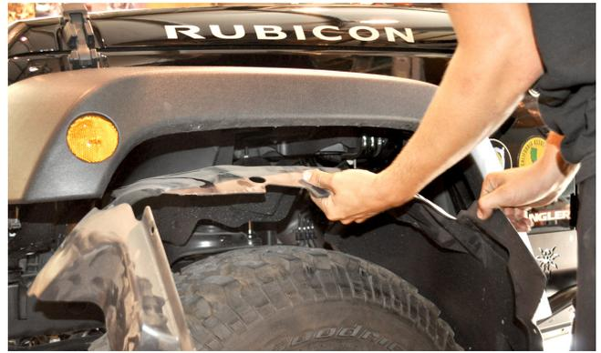
3. **Disconnect the side marker lamp** by pulling the wiring harness plug out of the lamp socket.
