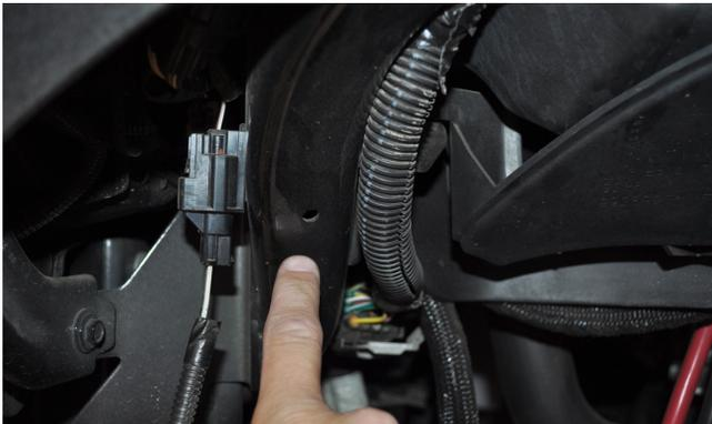
Transfer the location of this hole to the surface of the inner fender liner, mark and drill a corresponding hole with the 1/4" bit. Install one of the OEM plastic retainer clips at this location.
