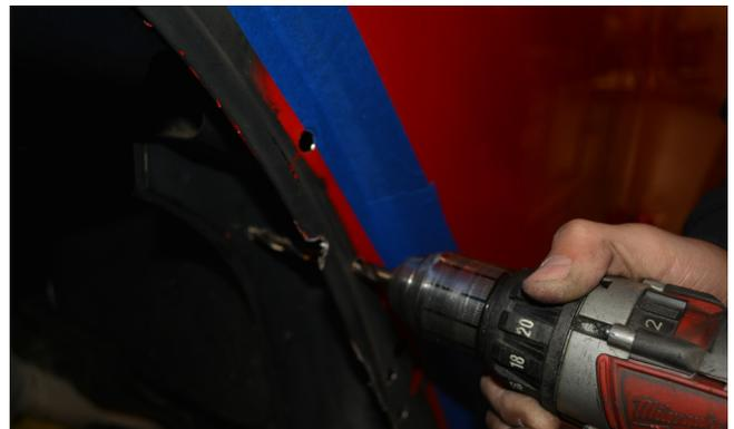
Use touch-up paint to coat the bare metal at the edges of the drilled holes, to prevent rust.
