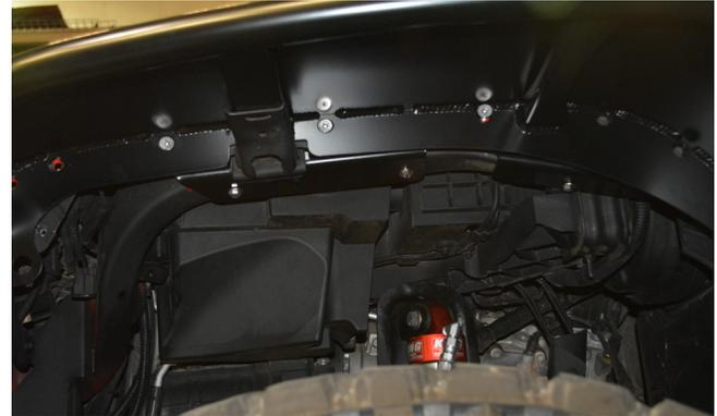
Install two of the 5/16-18 X 3/4 stainless steel flat head cap screws, one at the rear and one at the front end of the Crusher Flare. The one at the front will need to be backed by a flat washer and lock nut (supplied in the hardware kit)
