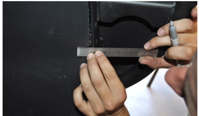
The inner fender liner is flexible plastic, and you will be able to pull it away enough to take your measurements. Mark the hole locations then drill the three holes with a 1/4" bit.
