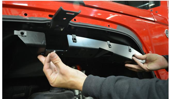
Re-use three (3) of the OEM metric hex head bolts to attach the Upper Sub-Frame Bracket, bolting them through the holes along the bottom of the bracket.
