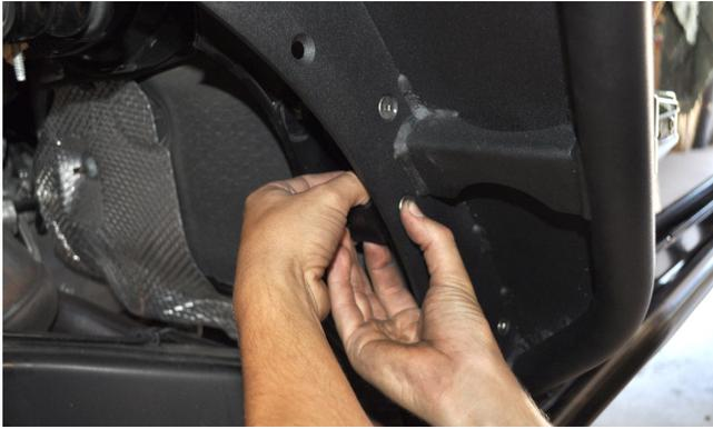
Adjust the "L" bracket so that the flat surface of the bracket and flush side of the U-Nut is parallel with, but recessed between 1/16" and 1/8" back from, the edge of the Crusher Flare mount plate. Tighten the lock nut on each bracket.
