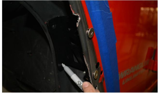
**18. Follow the same procedures as** in steps 9 and 10 to punch and drill the two holes in the inner tub brace. Drill the 1/8" pilot hole first, then step up to the 3/8" bit. You will have to pass the bit through the hole in the outer fender to reach the inner tub brace.
