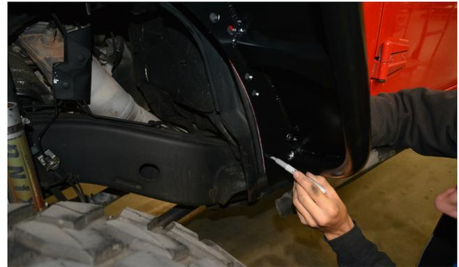
Continue installing hardware into the remaining available holes. Note the following diagram which shows the locations to use the 1" long flat head cap screws. The remaining holes get the 3/4" long flat head cap screws. (Note: several of the hole locations will need to be drilled out, and will not be able to accept hardware yet—leave these holes unused at this time.)
