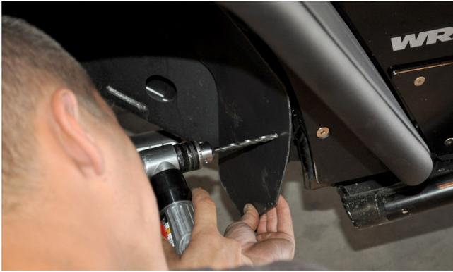
**29. Install a 1/4-20 X 3/4 SS Button Head Cap Screw with 1/4" SAE Flat Washer at each of the three holes that were just drilled in the previous step.** Insert the screw into the hole in the inner fender liner, and into the corresponding 1/4-20 U-Nut Clip that was installed in the "L" bracket in a previous step. Use a 5/32" hex key to firmly tighten each fastener. Be sure not to over-tighten and risk damaging the threads on the fasteners.
