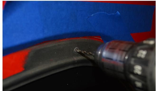
Once all of the pilot holes are drilled, switch to the 21/64" bit and re-drill each hole out to its final size. Be careful when drilling, as the larger bit may want to grab the thin sheet metal and deform it. After the holes are drilled, apply some touch-up paint or clear coat to the bare metal of the hole edges to protect them from rust.
