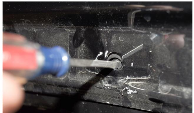
**20. Re-install the Lower Sub-Frame Bracket.** Use two 5/16-18 X 3/4 hex head cap screws with flat washers and nylon insert lock nuts to attach the bracket to the inner tub brace. Keep the holes in the bracket properly aligned with the holes in the outer fender as you tighten the bolts.
