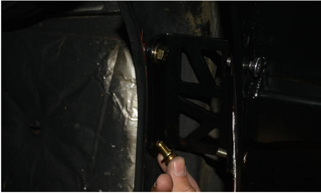
**21. If you wish to install** the supplied rubber gaskets, remove all but one of the flat head cap screws along the top edge of the Crusher Flare. Loosen the last screw enough to separate the Crusher Flare from the fender sheet metal slightly, but leave it engage enough to hold the flare on while installing the rubber gaskets.
