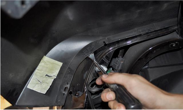
Some of these retainer clips are of a different type than the others, and are tougher to remove. Be careful when removing them not to bend or deform the Jeep body sheet metal. Set the stock fender flare aside. It will not be re-used.
