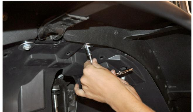
**28. At the rearward edge of** the inner fender liner, mark where the holes in the "L" brackets are located behind the inner fender.
