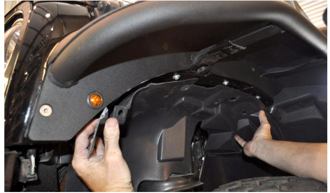
**27. Once the inner fender liner** is trimmed to fit, attach it by first removing the two previously-installed bolts from Upper Sub-Frame Bracket that appear through the access holes in the inner fender liner. Remove each of these bolts, place one of the provided 5/16 fender washers under the head of each, then re-install and tighten.
