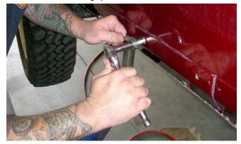
3. Once the nut-sert has seated correctly, loosen the bolt then remove it and the rest of the tool from the nut-sert. Install a new nut-sert onto the tool, oriented the same as the last, and set it aside until your next nut-sert installation.
