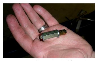
2. Use an open end wrench to hold the coupler nut stationary while turning the head of the bolt clockwise with a ratchet (or small impact wrench) and socket. As you turn the ratchet, the bolt will draw the far end of the nut-sert toward the inside of the sheet metal, gripping it with the knurled outside edge of the nut-sert as it deforms. Continue to turn the ratchet until the nut-sert is fully seated. DO NOT OVER-TIGHTEN as you can damage the nut-sert, or cause it to lose its grip.
