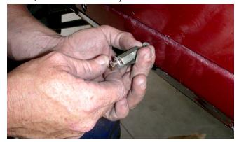
4. With the tool removed, inspect the nut-sert to make sure it is properly seated and that the surrounding sheet metal isn't excessively deformed. Note that some deformation of the sheet metal is normal, and that it will be covered by the part after installation.
