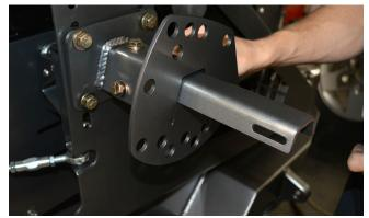
NOTE: Some tire/wheel combinations, such as 12.50 wide tires on stock Jeep wheels, may require more Overall Offset than the adjustment in the Tire Mount components allows (approximately 4-3/4" to 6-3/4"). In these cases, source a wheel spacer of suitable thickness to make up the difference.
