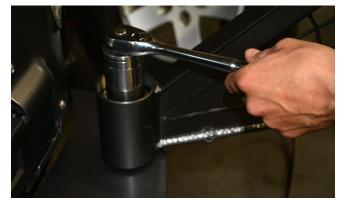
**22. Install the Pivot Cap O-Ring** onto the outside of the threads of the Billet Hinge Cap, just under the head of the cap (NOTE: this may have already been done prior to shipment).
