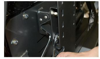
**28.** Assemble the Aluminum Turnbuckle, Spherical Rod Ends and SS Jam Nuts into a tie-rod assembly. Note that there are left hand threaded and right hand threaded ends of the turnbuckle, rod ends and nuts. (NOTE: the Turnbuckle Assembly may have already been preassembled at Poison Spyder). Use the provided hardware to attach one end of the tie rod to the Tailgate Plate, and the other end to the corresponding tabs in the back side of the Tire Carrier, as shown.
