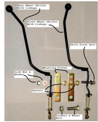
Verify parts required and pre-assemble the kit in this configuration.
