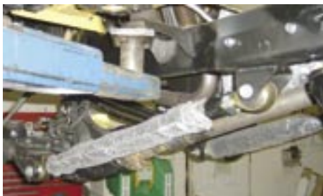
This photo shows the driver front arm and bracket properly installed.
