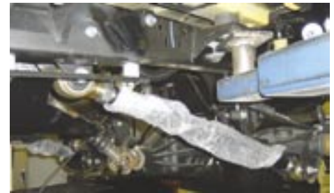
This photo shows the passenger front arm and bracket properly installed.
