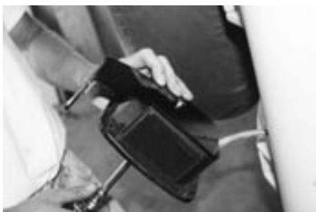
5. Locate the hole in the bracket directly above the tail light housing. Use a 1/4" bit to drill a hole through that hole and through the body. Use the
