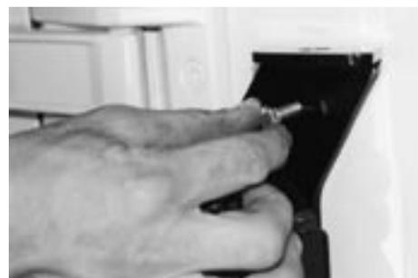
3. Position the antenna mounting bracket between the vehicle and the tail light housing. The mounting portion of the bracket will be positioned towards the outside edge of the tail light housing when properly installed.
