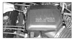
3. Loosen the bolt on the resonator as shown.
