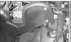
8. Install the heat shield into the vehicle and secure the twist bracket to the original air cleaner mounting hole using the provided hardware.
