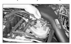
12. Connect the provided hose to the vent on the valve cover, then, connect the other end to the vent on the K&N intake tube as shown.
