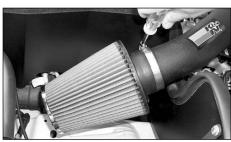
13. Install the K&N Filtercharger onto the K&N intake tube and secure with the provided hose clamp.
