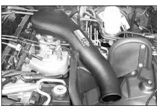
11. Install the K&N intake tube into the silicone hose as shown, but do not tighten completely as some adjustment may be necessary.
