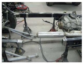
13. Prepare the frame extension pieces. The extensions come E-coated to prevent corrosion. This is the same coating the rest of the frame comes with from the factory. Grind the edges with a 45 degree bevel and remove any excess paint. Using the tape measure, combination square and scribe, mark the inside center of each extension with the tube seam to the inside of the frame. You'll use this to help align the fishplates later on.
