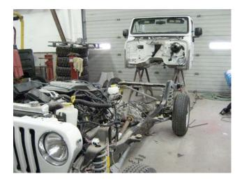
4. Remove the brake and fuel line bundle. Rubicon Locker Pump hose and any vapor lines on your particular year Wrangler will be lengthened with rubber hose available at any auto parts store. Be sure to get hose that is not affected by gasoline fumes for any vapor lines.
