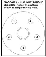
**WARNING:** Retighten lug nuts at 500 miles after any wheel change, or anytime the lug nuts are loosened. Failure to do so could cause wheels to come off while vehicle is in motion.
