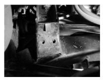
**Step 1:** Take the T-shaped plate with integral nuts and slide it into the driver's side motor mount through the top opening. Once the nuts can be seen through the two holes in the lower side of the motor mount, the tab may be folded over to hold the nuts in position. It is helpful to give the tab a slight arch before inserting it into the motor mount.
