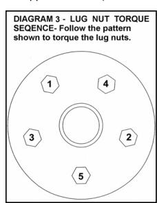
WARNING: When the tires / wheels are installed, always check for and remove any corrosion, dirt, or foreign material on the wheel mounting surface, or anything that contacts the wheel mounting surface (hub, rotor, etc.). Installing wheels without the proper metal-to-metal contact at the wheel mounting surfaces can cause the lug nuts to loosen and the wheel to come off while the vehicle is in motion.
