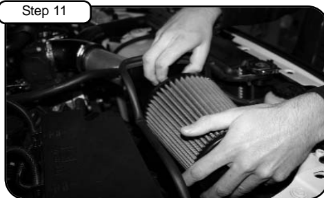
Step 11 Re-install Crankcase line to new tube with mini clamp provided and tighten using 1/4" nut driver. Place high FLOW filter into housing and tighten using 5/16" nut driver.
