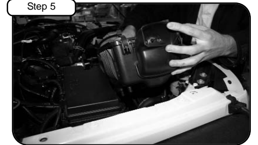
Step 5 Carefully pull out bottom half of airbox. ( caution, this may require some force )
