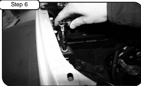
Step 6 Loosen 10mm bolt holding in airbox bracket.
