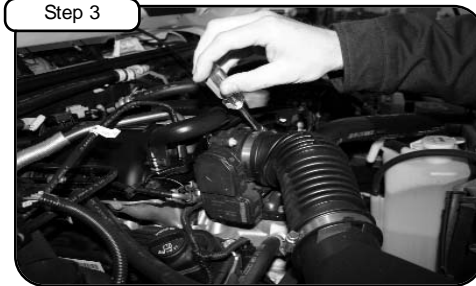
Step 3 Loosen clamp using 5/16" nut driver @ Throttle body.
