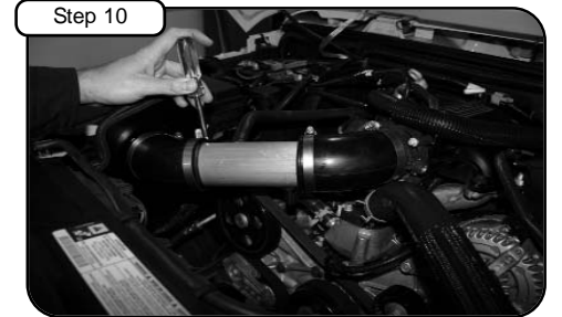
Step 10 Install 3" end of coupler to housing side and 2 3/4" coupler to throttle body side. ( make sure temp sensor side of tube is near throttle body side ) Tighten clamps using 5/16" nut driver.
