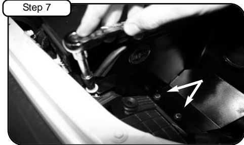
Step 7 Install trim seal to housing and place in to vehicle. Retighten bolt from step 6. With screws provided, tighten down both bolts using 9/16" socket or wrench.
