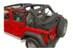
The outer protective bag should fit snugly around the window roll felt as not to cause any flapping. During hot weather the windows may flatten some on top. This is considered normal and does not harm the windows. Check the buckles from time to time to insure the bag is secure.
