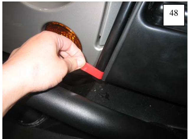
Pull tape liner from tape and press part to secure tape. Tighten all Truss Head Screws first, then tighten Torx Screws, moving from back to front.
