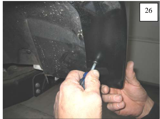
Replace splash shield, and install a supplied Truss Head Screw through rearmost hole in flare and into clip installed in Step 25. Reinstall three pocket screws removed in Step 24.
