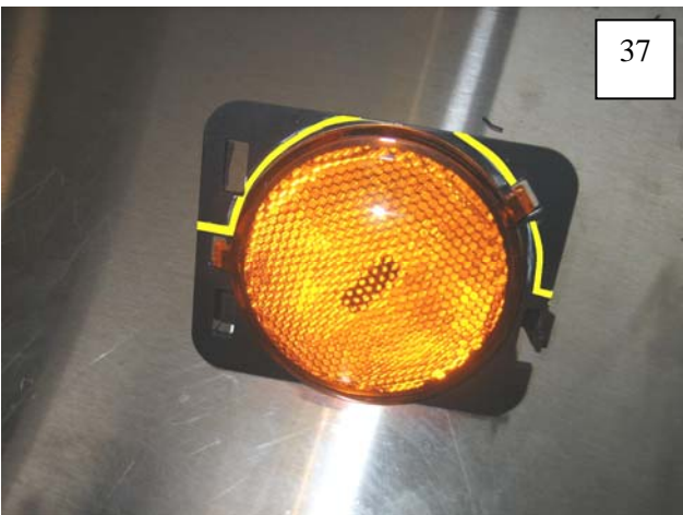
Carefully cut or grind factory light bezel along lines shown. Take care not to cut light lens.
