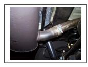
2. To remove the stock exhaust, unbolt band clamp located just behind your factory muffler. Disengage the welded hangers using WD-40 from the OEM rubber grommets. Do not damage or remove the rubber grommets as you will reuse them to mount your new system. Now, cut off tailpipe and remove exhaust.
