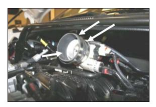
12. Install the provided reducer (#6) onto the throttle body with the smaller diameter towards the throttle body. Place the #48 hose clamp (#13) on the smaller diameter section of the reducer (throttle body side). Place the #52 hose clamp (#14) on the larger diameter side of the reducer. Leave the clamps loose for now.
