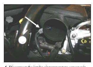
**6.** Disconnect the intake air temperature sensor wiring harness, by squeezing the tab on the side, and sliding the connector off.
