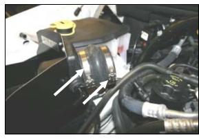
**13.** Install the urethane hump hose (#7) onto the air filter adapter using two #60 hose clamps (#15) on each side of the hump hose. Tighten <u>only</u> the clamp on the air filter adapter. Leave the other clamp loose for now.
