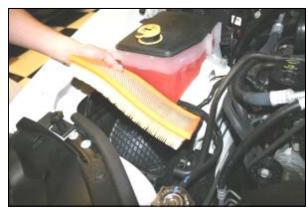
**5.** Remove the factory air filter.
