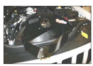
**9.** Assemble the Quick Fit panels (#2, #3) as shown, using five 6-32 screws (#16), #6 flat washers (#17), and 6-32 keps nuts (#18).
