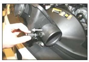
**14.** Remove the factory intake air temperature sensor from the resonator box by carefully twisting the sensor body, and pulling it straight out of its mount. Place the sensor in a safe location, it will be re-used in step #15.
