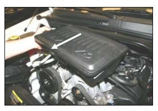
**8.** Remove the factory intake resonator box from the throttle body by pulling the box towards the radiator and then lifting up.
