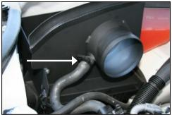
in the bottom of the stock air box by sliding the four tabs on the back into the slots on the airbox, once installed, re-hook the two latches. Next, install the speed clamp over the breather hose and connect it to the Quick Fit assembly as shown.
