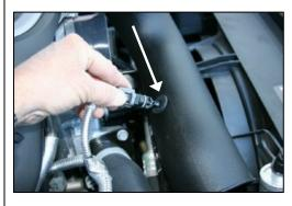
**17.** Carefully install the temperature sensor into the grommet. Make sure it goes all the way in.
