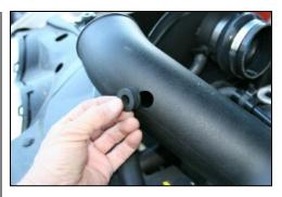
**16.** Install the supplied grommet into the hole in the back of the tube.
