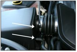
1. Disconnect the negative battery cable. Loosen the hose clamp on air cleaner box lid. Twist and remove breather hose from air cleaner box lid.
