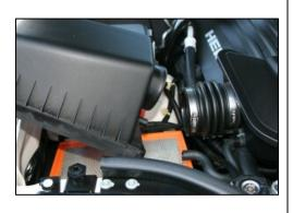
3. Remove the air cleaner box lid by sliding it forward, and then up, and out of the factory intake tube.
