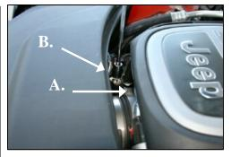
**7.** A.) Loosen the hose clamp on the throttle body. B.) With a 10mm socket, remove the bolt next to the throttle body that holds the intake resonator in place.
