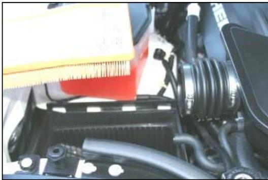
**4. Remove the factory air filter from the airbox base.**
