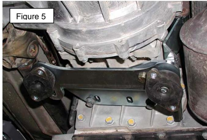
removed. This will be easiest if you increase the height of the jack under the transfer case output so that the trans is higher relative to the exhaust than it was stock. Start *all* bolts by hand, then torque to 50 ft-lbs. **Figure 5** shows a mount installed on a TJ Rubicon with 4-speed automatic – others will look similar.
