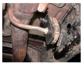
**Step 17:** Place the Exhaust Hanger Adjuster over the exhaust hanger pins as shown in the photo to the left. This "locks" the two pins together to facilitate bending the frame mounted pin upward in the next step.
