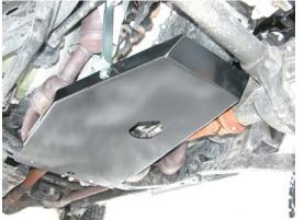
**Step 7:** Using a floor jack (or a friend) position the skid plate as shown at left.
