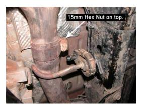
**Step 16:** Loosen one of the bolts that holds the exhaust Y pipe to the exhaust manifold on the passenger side. We have found that the front-most bolt is most easily accessed from the inner fender area. Again, there is no need to loosen both bolts.
