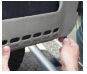
(4) Insert one end of new Nylon door strap through the front slot of the inner door skin. With hand Inserted into door from underneath align eyelets with threaded clip. Make sure not to dislodge clips. If this happens, simple reinsert and continue with installation. With handle ends installed push panel back and secure strap with screws saved in step (2).
