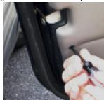
(2) remove screws securing pull handle to door. Keep screws as they will be reused.
