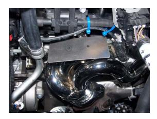
4. (NOTICE IN PICTURE) THERE IS SUPPLIED HEAT SHIELD TO BE CLAMPED ON MIDDLE HEADER TUBE. THIS WILL PREVENT HEAT GOING TO COIL PACK ABOVE HEADER ASSEMBLY. NOW RE-INSTALL STEERING SHAFT USING RED LOCKTITE BEFORE TORQUING FASTENER.
