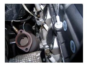
6. NOW INSTALL GIBSON HEADER WITH SUPPLIED GASKET RE-USING STOCK BOLTS TORQUING TO 30-35 FT-LBS FROM CENTER OUT. AFTER HEADER IS IN PLACE, USE SUPPLIED HEAT WRAP ON SPARK PLUG WIRES AND ZIP TIE TO KEEP AWAY FROM HEADER FOR HEAT PROTECTION. (NOTE: MAKE SURE ALL WIRES AND HOSES HAVE PROPER CLEARANCE FROM HEADER!)
