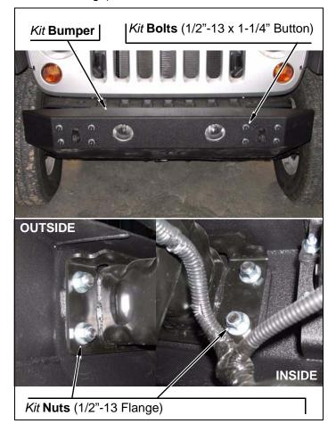
6. Install kit bumper onto lower crush zone with four kit nuts (1/2"-13 Stover), four kit large washers (1/2" ID), and four kit bolts (1/2"-13 x 1-1/4" button). TIGHTEN all kit bumper hardware.
