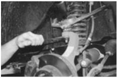
13. Use a 21mm wrench to remove the nut that secures the ball joint of the A-arm to the top of the knuckle.
