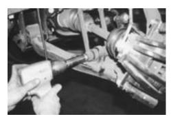
14. Use a 21mm socket to remove the nut that secures the fork to lower A-arm assembly.
