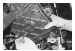
11. Disconnect the battery sensor from the bottom of the battery tray.
