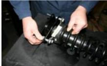
20. Lift the strut assembly into position. Attach the four top nuts using the new nuts and washers. Reassemble the fork to the bottom of the strut.
