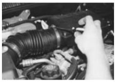
3. Loosen the hose clamps to remove the air box from the air intake hose.
